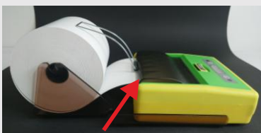
Insert the paper into the gap between the cabinet and the paper cover.
